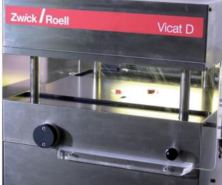
heating block at the pre-set rate is started. When the required penetration is reached at all stations, the heating is switched off and the test is ended.
