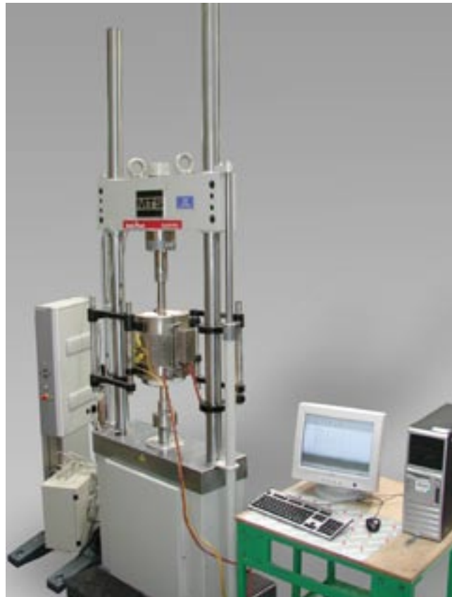
Modernized MTS 1S with testControl
