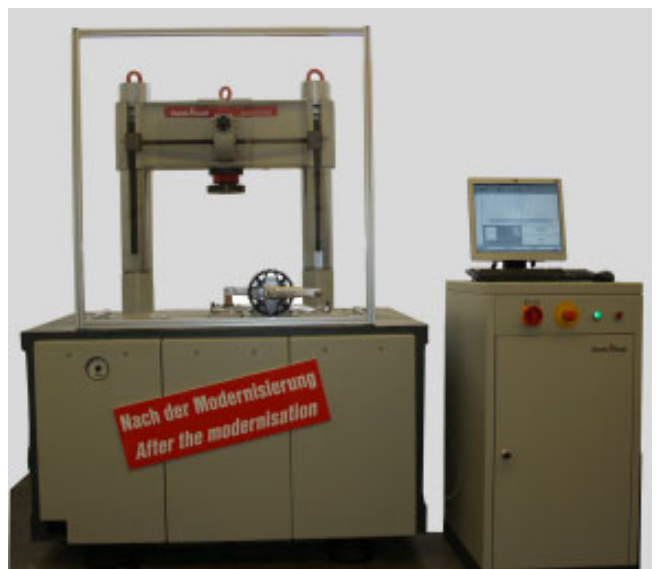
Modernized Schenck unbalanced mass pulsator
