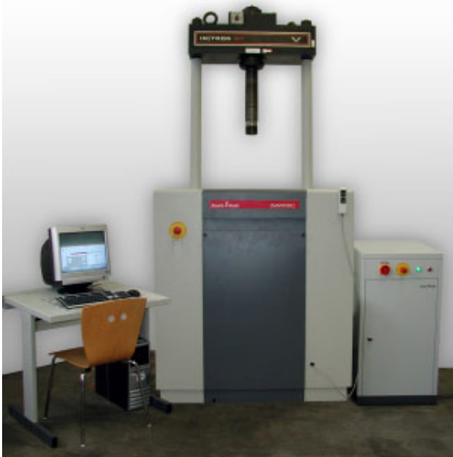
Modernized Instron Pulsator Type 1603
