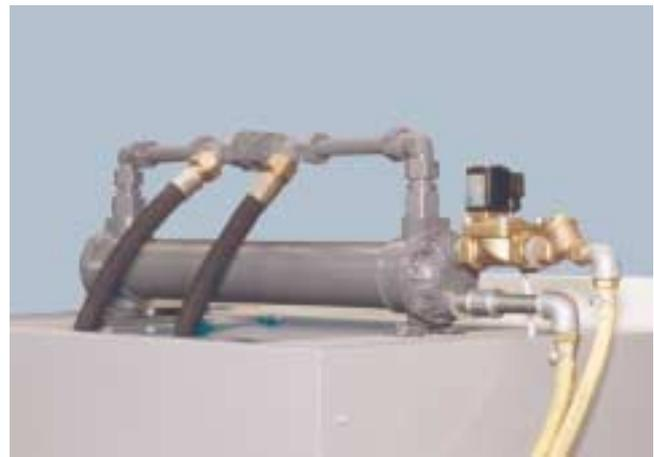
Fig. 06: Optional water heat exchanger
