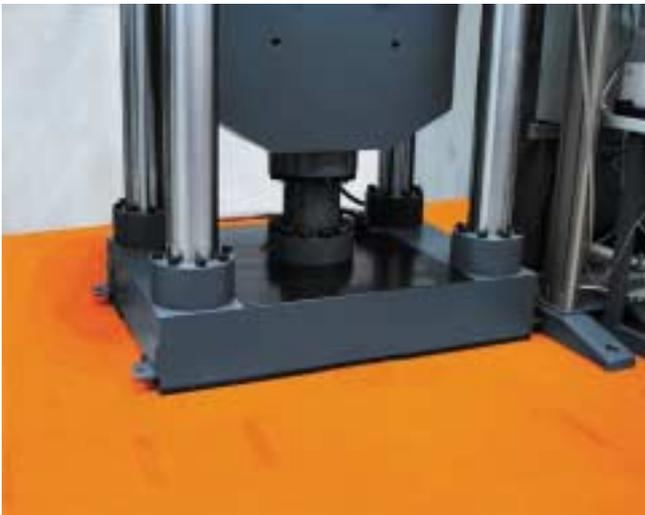
Fig. 05: SP Machines do not require foundations
