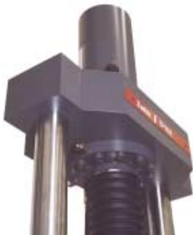
Fig. 03: Zwick SP600 load frame with fixed crosshead
