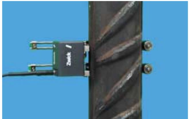
Fig. 14: Zwick extensometer Digital Clip-On with extension pieces for large diameters
