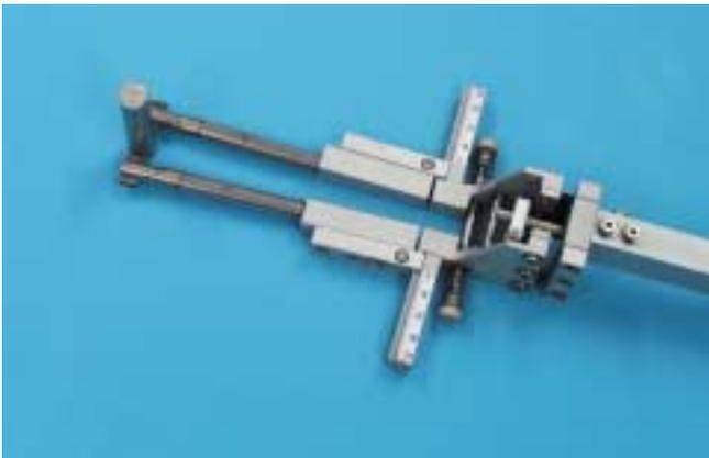
Fig. 12: Sensor arms for SP-Macro for sample diameter / thickness up to 110 mm (example with small diameter, BSP066550.20-003)
