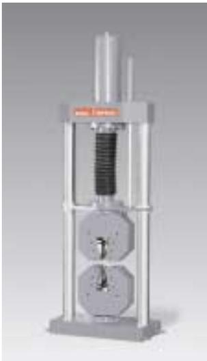
Fig. 01: Zwick SP600 load frame; 2 columns, crosshead fixed
