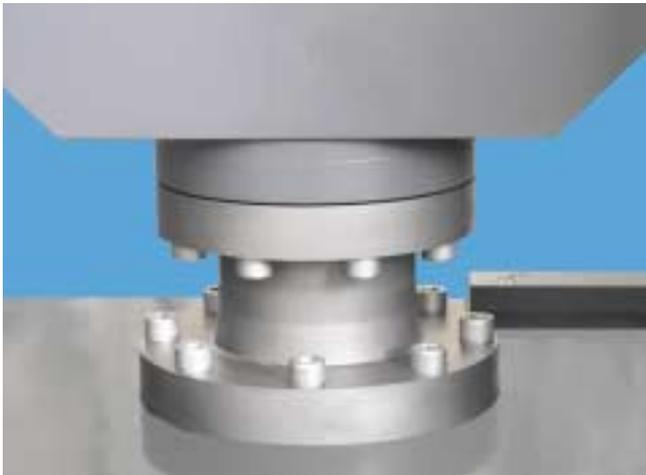
Fig. 07: Electronic load cell for SP Machines
