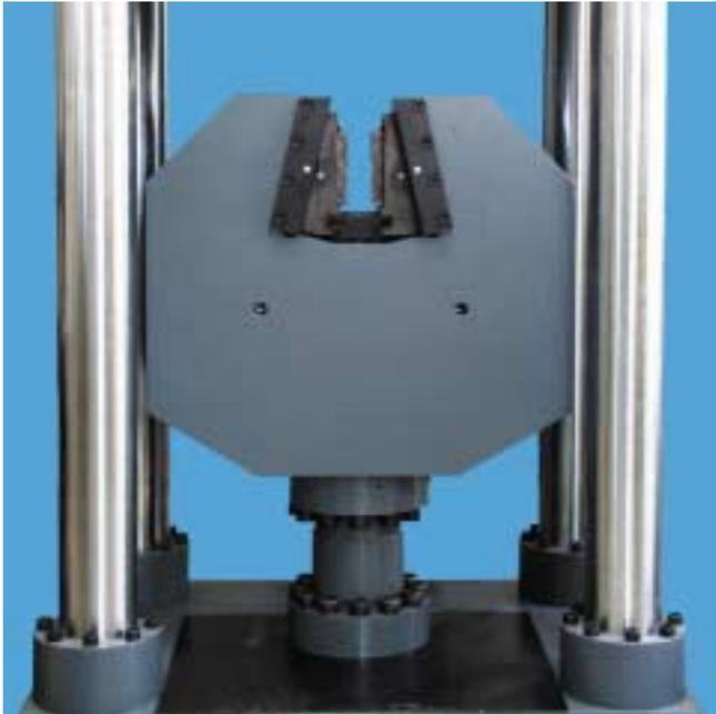
Fig. 15: Lower grips 2000 kN with open front design
