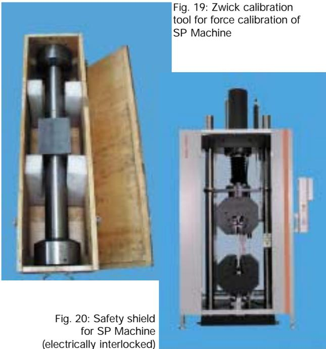
Fig. 19: Zwick calibration tool for force calibration of SP Machine
