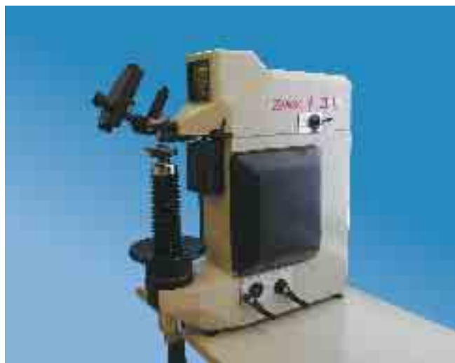
Fig. 14: The Zwick/ZHU 187,5 universal hardness tester is available in a range of designs and for a range of different test load combinations
