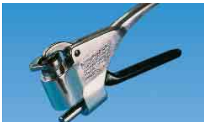
Fig. 19: The Webster Portable hardness tester
