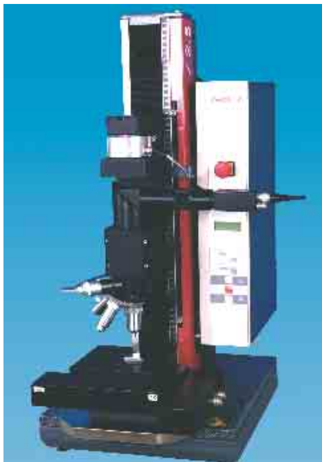
Fig. 9: The Vickers hardness testing machine ZHV20/Z2,5
