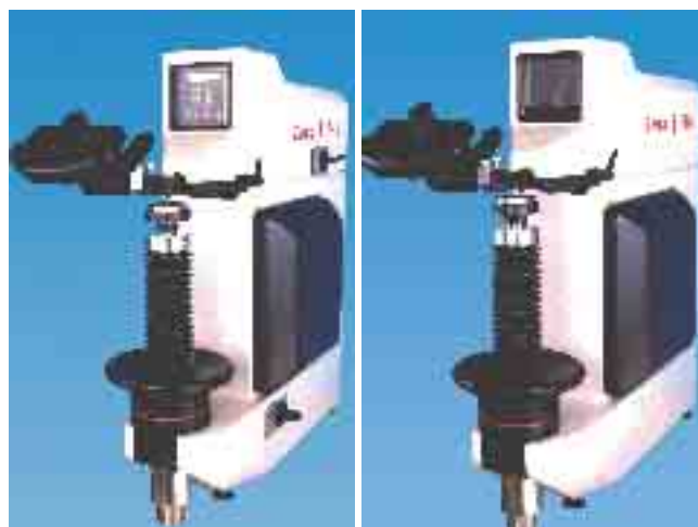
Fig. 13: The Vickers hardness testers Zwick/ZHV 30 (left) and Zwick/ZHV 50 (right); the testers differ to the extent of their load stages, the type of load change and some software functions
