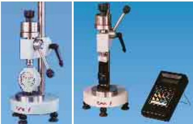
Fig. 21: The Zwick 3114 with test stand Fig. 22: The digital Shore hardness tester Zwick 3140
