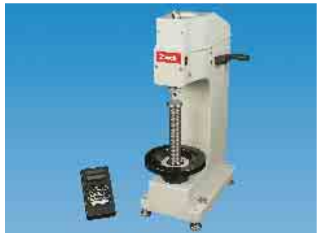
Fig. 17 The Zwick 3106 – The ball indentation hardness tester from Zwick
