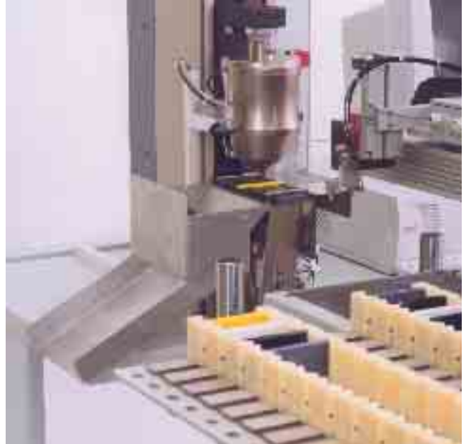
Fig. 6: The Zwick hardness measurement head with automatic specimen feed will be put to use for fully automatic hardness tests on plastics
