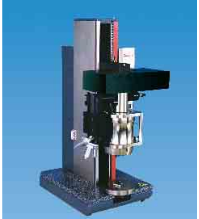
Fig. 11: The Universal hardness testing machine ZHU2,5/Z2,5 with supplementary unit "Optic"
