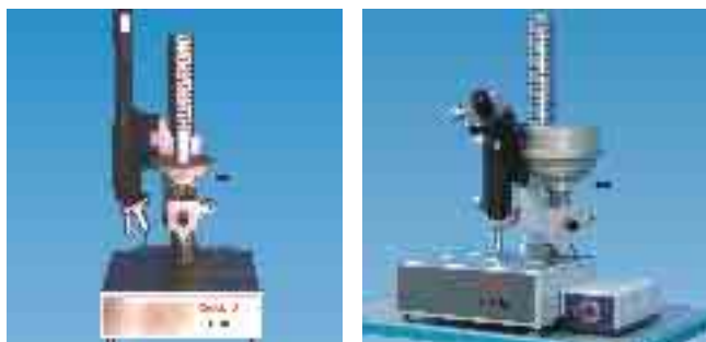
Fig. 12: The Vickers hardness tester Zwick/ZHV 10 (left: Analogue version, right: PC version)
