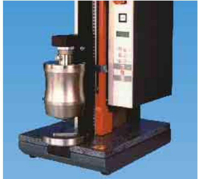
Fig. 4: The Zwick hardness measurement head is used for hardness tests on metals
