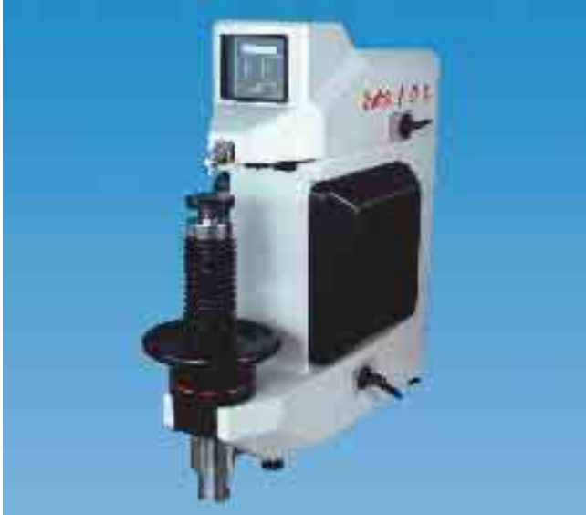
Fig. 16: The Zwick/ZHR 8150LK for series tests with small batch sizes
