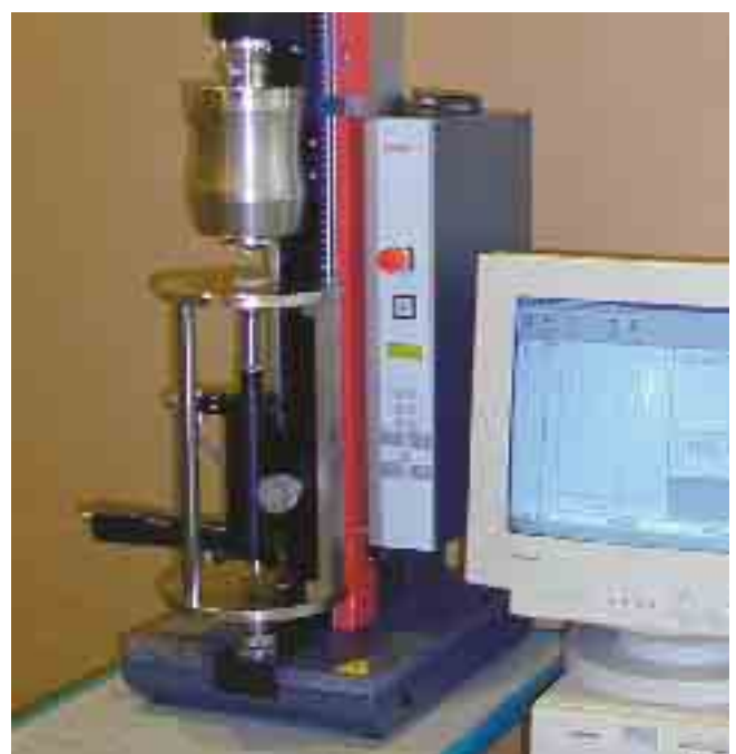
Fig. 8: The ZHU0,2/Z2,5 is used for tests on glass
