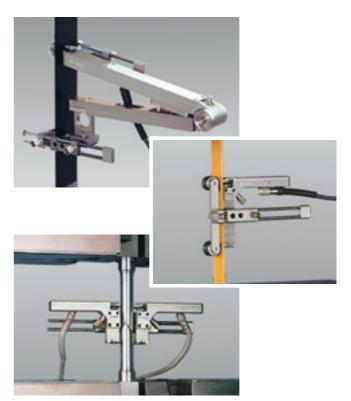
Fig. 19: Strain gauge clip-on extensometers
