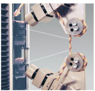
Fig. 23: The optical extensometer for non-contact measurement
