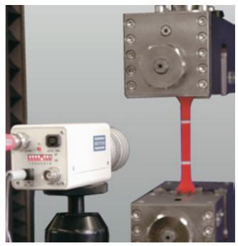
Fig. 27: The specimen surface is digitalised by a full-frame camera
