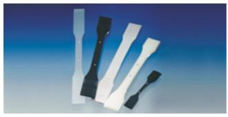
Fig. 22: Marked specimen for optical measurement
