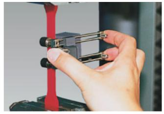
Fig. 12: The incremental clip-on extensioneter guarantees simple and rapid handling.
