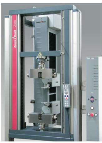
Fig. 8: The universal extensometer multiXtens
