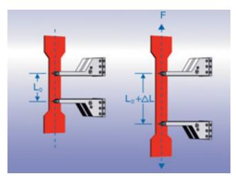
Fig. 3: Direct extension measurement
