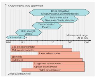
Diagram 3: Range of application of Zwick extensometers dependent upon the measurement travel
