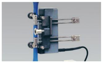
Fig. 14: Incremental clip-on extensometer (TC-EXICLEL.002)
