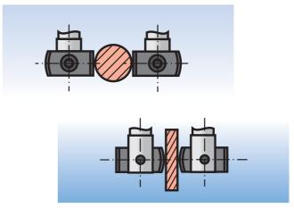
Fig. 5: Round specimen with straight knife edges, and flat specimen with convex ones
