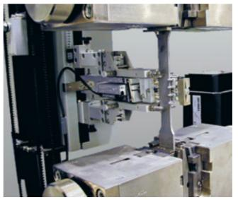
Fig. 10: Macro extensioneter in combination with a reduction in width monitor (With 4 measurement lines)
