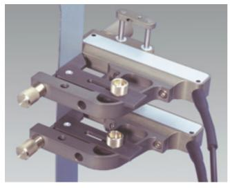
Fig. 18: Strain gauge clip-on extensometer for width measurement
