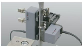
Fig. 16: Biaxial incremental clip-on extensometer
