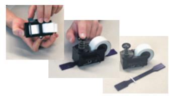
Fig. 26: The specimen marking devices are simple to operate and are functionally safe (Here a simple manual device)
