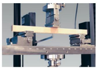
Fig. 20: Extensometer for 3-point flexure test
