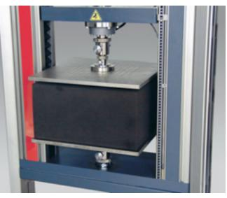
Fig. 2: The extension is measured indirectly at this compression test
