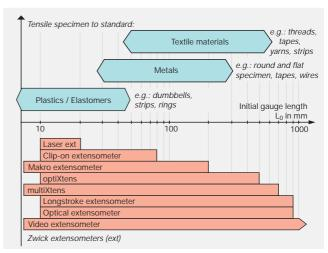
Diagram 2: Application range of Zwick extensioneters dependent upon the initial gauge length  ${\rm L_0}$
