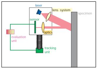
Fig. 29: optiXtens (Upper measurement head) setup and principle of tracking the reference speckle
