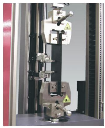
Fig. 11: Longstroke extensometer
