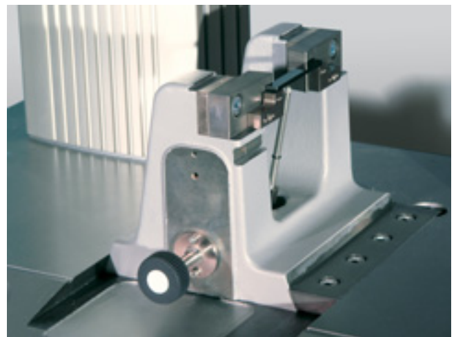
Fig. 3: Instrument base and gripping wedge of the impact support
