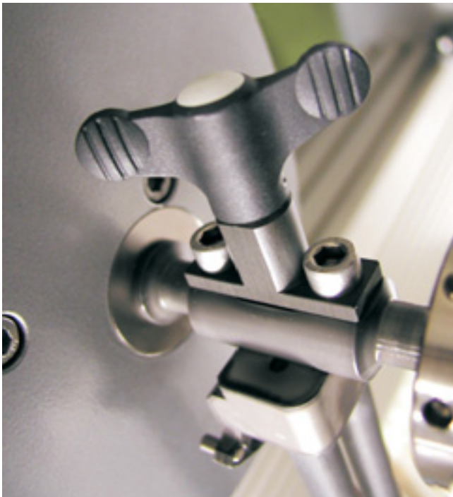
Fig. 1: Pendulum quick release for fast changing of pendulums
