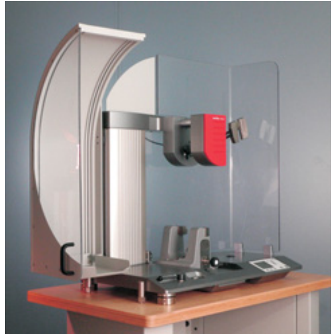
Fig 1: Pendulum Impact Tester HIT5.5P
